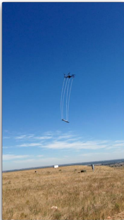
Figure 1. Conventional UAV aeromagnetic survey flying near the Boulder Magnetic Observatory outside of Boulder, CO.
